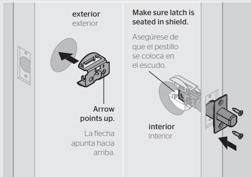
**Latch shield must be installed to maintain fire rating.**
