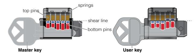
In fact, since every pin location has 2 shear lines and there are 5 pin locations in this cylinder, there are:
