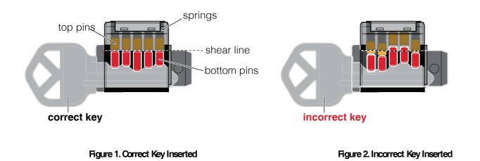
Alternatively, when another key with a different key cut is introduced, the pins are pushed up, but do not create the shear line and therefore the cylinder cannot be engaged.
