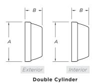
780,782 Interior 45mm 64mm 24mm 780,782 Exterior 67mm 29mm 784,785 Interior 67mm 29mm 784,785 Exterior 67mm 29mm
